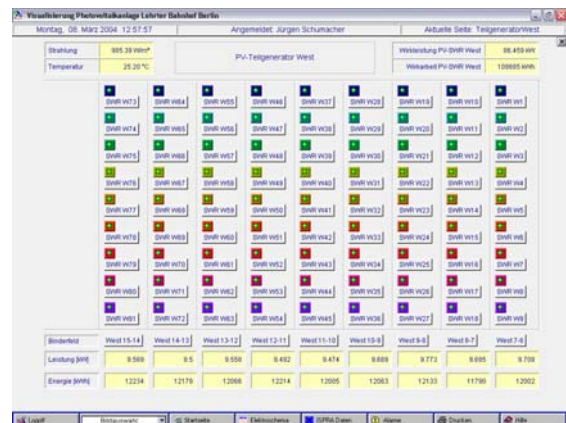
Figure 3: Detailed view of the west side generator of the main railway station project in Berlin with operating indicators for each individual inverter and visualisation of power and energy of each roof row.
