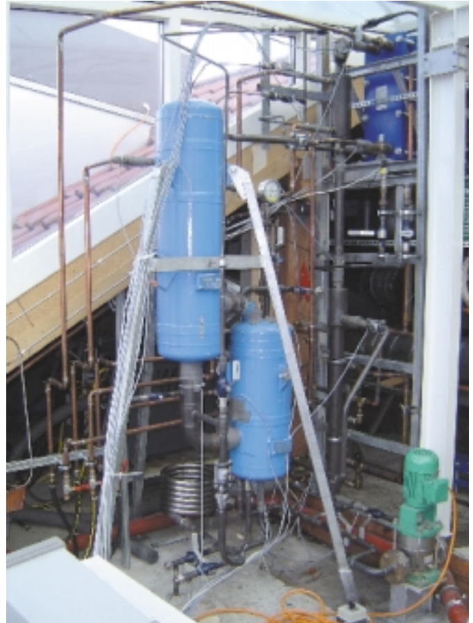
Near-market prototype DACM produced in the laboratory of the Stuttgart University of Applied Sciences ULI JAKOB HFT STUTT GART
