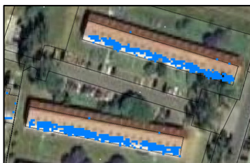
Picture 8: Result of the intersection of the inclined roof inclination and orientation
