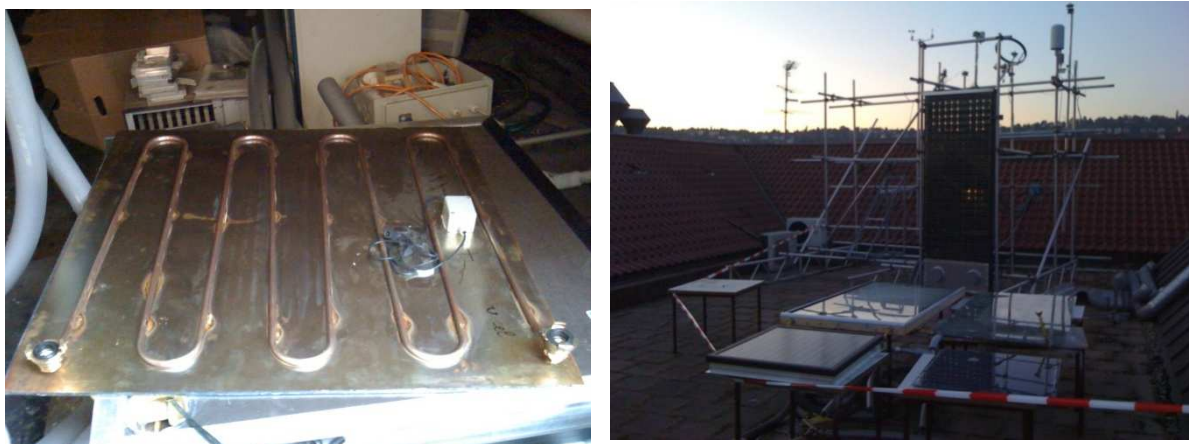
Figure 2: PVT collector (PVTwins) and experimental set-up
