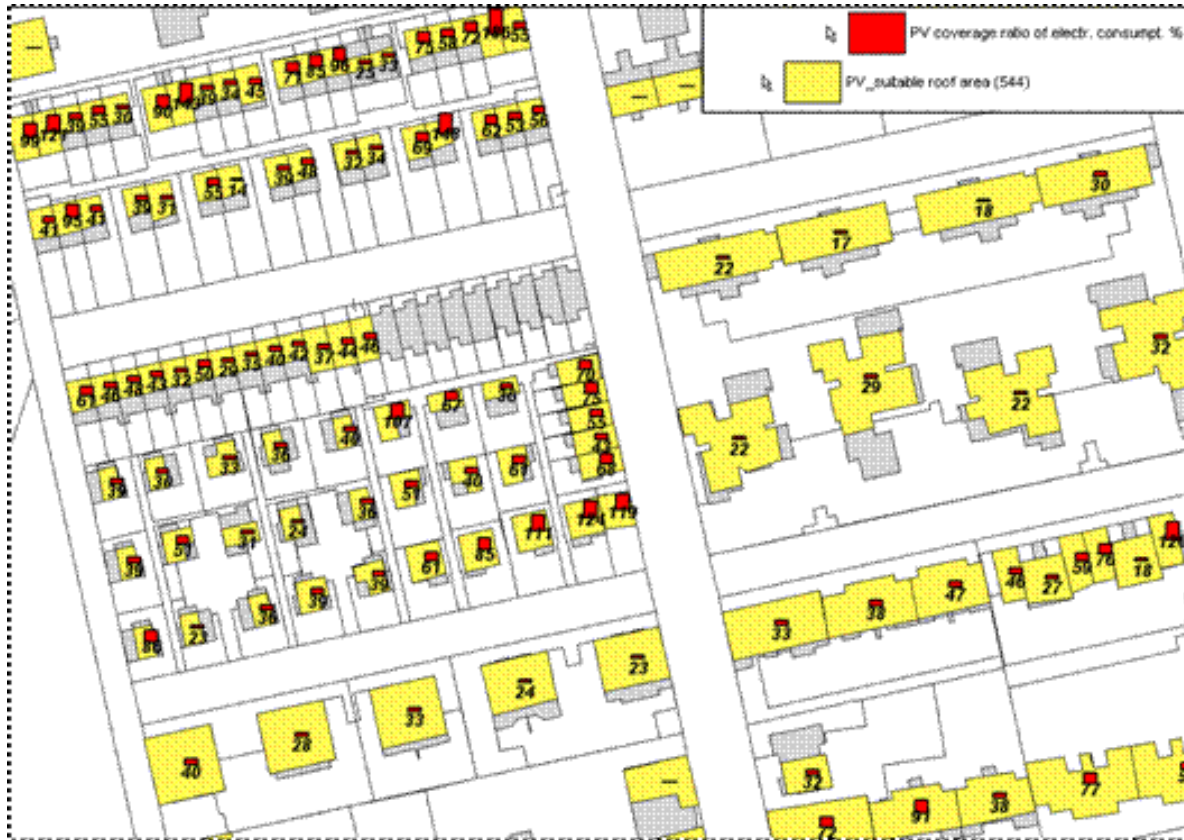
Figure 8: Representation of suitable roof areas and percentage of PV coverage per building.
