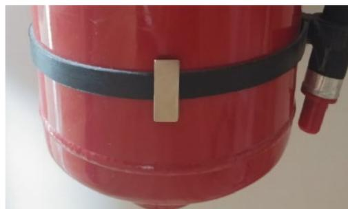
Figure 8. Contact sensor attached to a fire extinguisher
